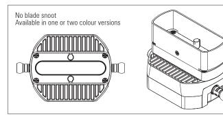
Two colour snoots - The finish of the interior louvre section can be different from the outer finish of the fixture. E.g. white exterior body finish with black interior louvre section
